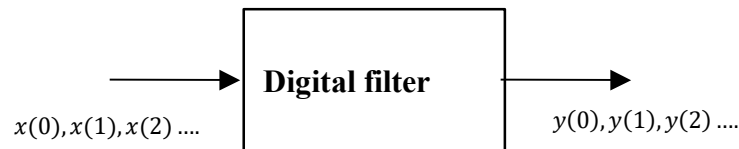
Figure 1.5: Representation of an Input-Output Relationship in a Discrete-Time System
